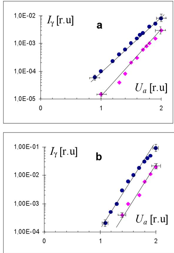
Fig.2. The light radiation intensity ( $I_\gamma$ ) vs RF power ( $U_a$  is the loop signal) for two types of cavities: space homogeneous (a) and space inhomogeneous (b) RFQ.
