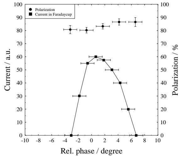
Figure 6: Phase resolved measurement of the polarization of the electron bunches. The spin polarization (upper points) and the transmitted current (curve on the bottom of the plot) are shown as a function of the deflector cavity phase.
