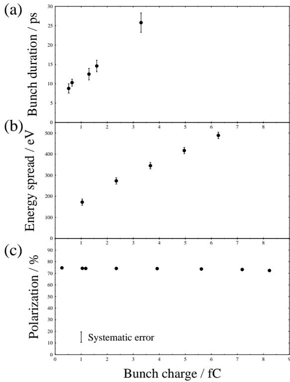
Figure 5: Polarization, bunch duration and energy spread of the bunches vs. the bunch charge. These three measurements were not taken at the same time. The strong dependence of the bunch duration on the bunch charge is considered to be an external space charge effect.
