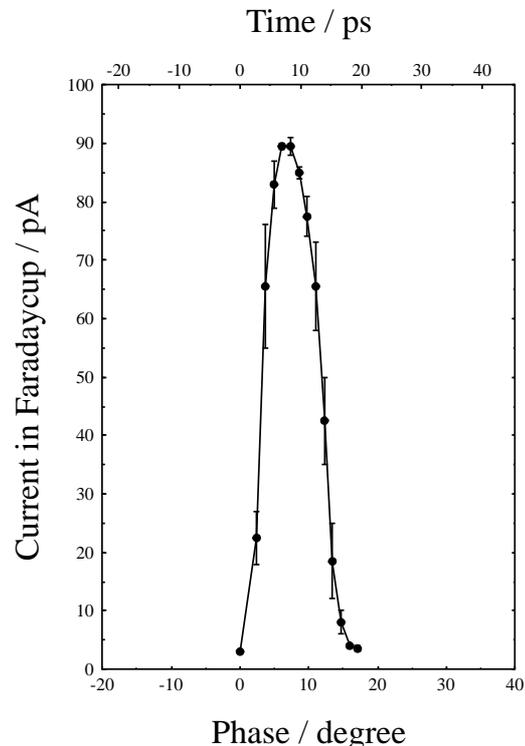
Figure 4: (a) An electron bunch generated with an accelerating voltage of 100 kV at a quantum efficiency of  $5 \times 10^{-4}$ . To guide the eye, the points are connected with straight lines.
