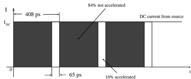
Figure 1: The transmission of the d.c. source current through the accelerator. At best 16% of the generated electrons reach the experiment.
