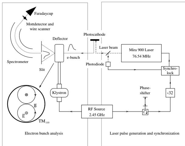
Figure 3: Principle of the measurement is a radiofrequency streak method. On the right side the laser pulse generation and synchronization to the MAMI rf is shown. The left part of the sketch shows the electron bunch analysis with the  $TM_{110}$  deflector cavity.
