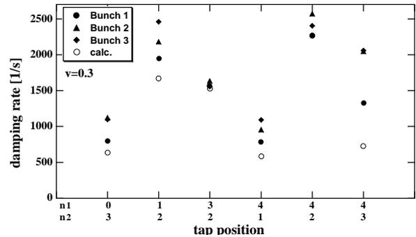
Figure 7: The damping rates of the experimental results and the calculations in 3-bunch operation with  $\nu=0.300$ .
