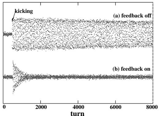
Figure 3: The observed oscillations with feedback off (a) and with the feedback on (b). The transverse oscillation was excited by a kicker magnet for the injection.
