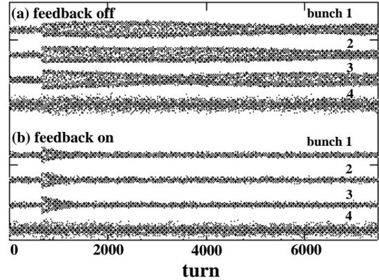
Figure 6: The observed oscillations with feedback off (a) and with the feedback on (b) in 3 bunches. Bunch 4 is absent in this data.
