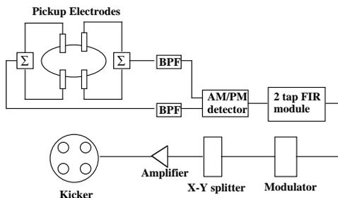
Figure 2: Block diagram of the feedback system.
