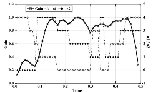
Figure 1: The graph of the maximum net gain and the tap-position as function of  $\nu$ . The maximum tap-position is restricts to 4.
