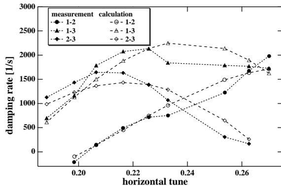
Figure 5: The damping rates as functions of tune along  $\nu=0.235$ . The data were taken for several tap-positions. In the figure, for example, 1-2 means the tap-position of  $n_1=1$  and  $n_2=2$ .
