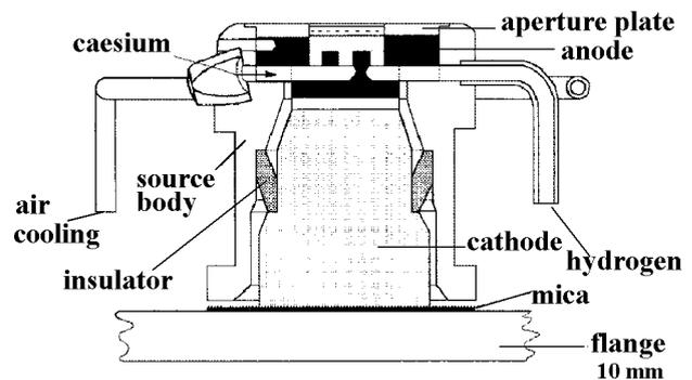
Figure 1. Schematic of ISIS H<sup>-</sup> ion-source
