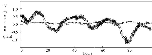
**Figure 1** Vertical orbit motion at one BPM over 4 days with and without feedback. Step changes occur after each fill and energy ramp cycle.
