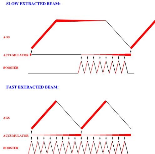
Figure 4: A 1.5 GeV accumulator in the AGS tunnel can be used for both slow-extracted beam (SEB) and fast-extracted beam (FEB) to improve the machine duty cycle. Operation scenarios for these two modes are shown with the thickness of the line indicating the beam intensity.
