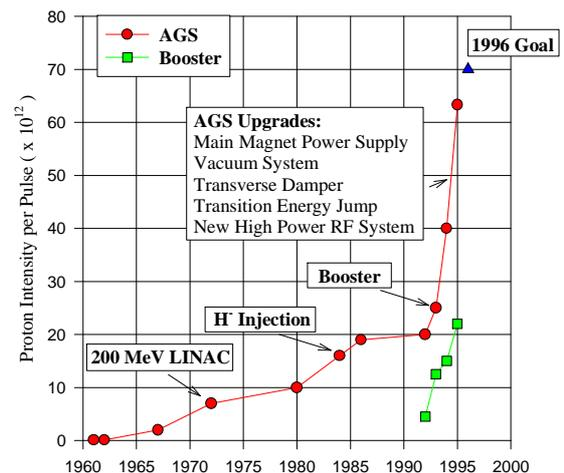
Figure 1: The history of the evolution of the proton beam intensity in the Brookhaven AGS.
