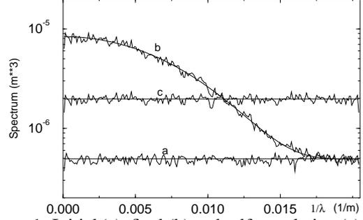
Figure 1: Initial (a), final (b) and self correlation (c) spectra for one to one correction by steering,  $\sigma_{\text{ini}} = 100 \mu\text{m}$ . All spectra on pictures doubled in comparing with formulae.
