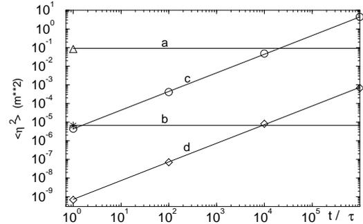
Figure 2: Dispersive error for the “one-to-one” correction by steering, a) and b)  $\sigma_{\text{ini}} = 100 \mu\text{m}$ ; c) and d)  $AtL = 10^{-12} \text{ m}^2$ , before and after correction.
