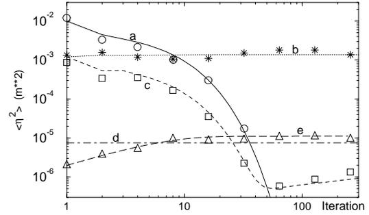
Figure 4: Dispersive error for ‘‘adaptive alignment’’. a)  $\sigma_{\text{ini}} = 100\mu\text{m}$ ; b)  $\sigma_{\text{res}} = 10\mu\text{m}$ ; c)  $\sigma_{\text{off}} = 10\mu\text{m}$ ; d) the limit at  $n \rightarrow \infty$  of the case c); e)  $A\Delta tL = 10^{-12} \text{m}^2$ .
