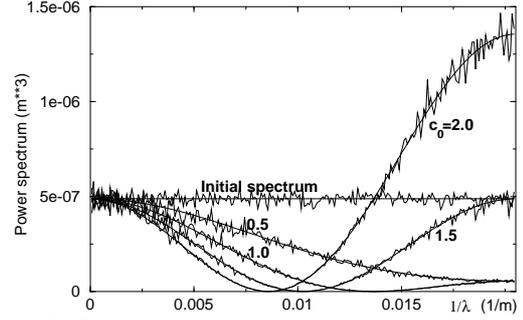
Figure 3: Power spectrum after first iteration of the ‘‘adaptive alignment’’ for different  $c_0$ ,  $\sigma_{\text{ini}} = 100\mu\text{m}$ .
