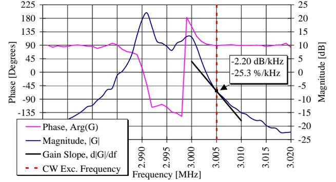
Figure 1: Longitudinal BTF measured in the PSB
