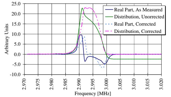
Figure 2: Measured real part of longitudinal BTF and its integral the density distribution  $\Psi(f)$
