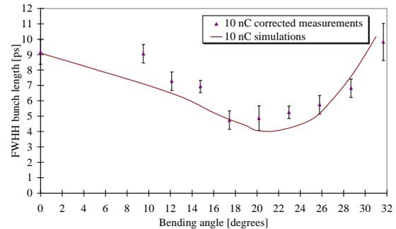
Figure 4: Compression of a 10 nC bunch
