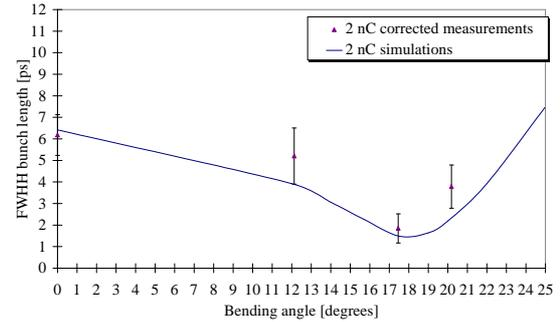
Figure 3: Compression of a 2 nC bunch
