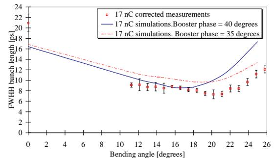
Figure 5: Compression of a 17 nC bunch
