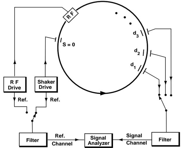
Figure 1: Schematic illustration of the experimental setup.
