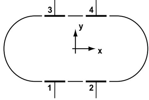
Figure 2: Beam button layout at a detector.
