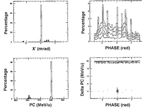
Fig.4. Simulation of RF stacking for  $^{132}\text{Sn}^{50+}$  with electron cooling and stochastic cooling
