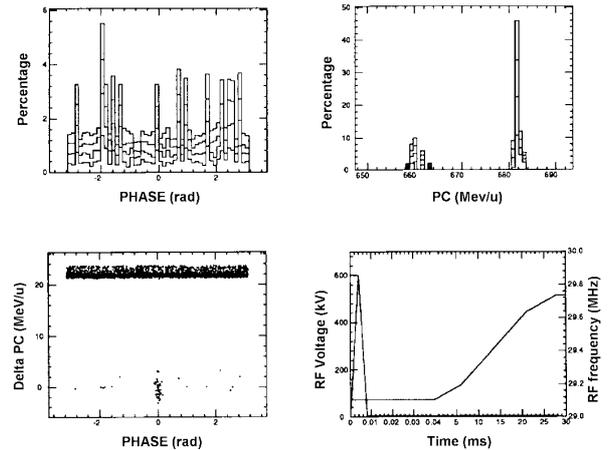
Fig.1. Simulation result of RF stacking for  $^{132}\text{Sn}^{50+}$
