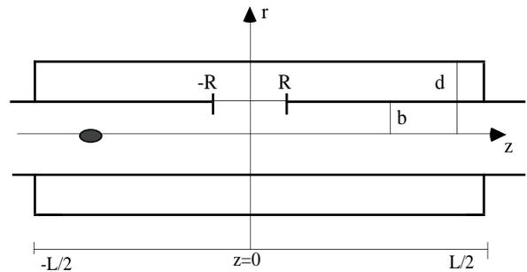
Figure 2 : Coaxial resonator.
