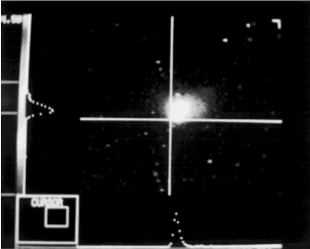
Figure 4. Electron beam spot at Linac end. The energy is 510 MeV and the sigma is  $\sim 1.5$  mm.
