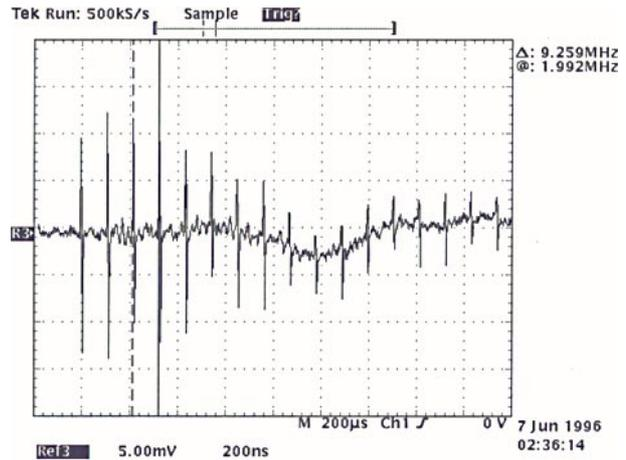
Figure 5. Circulating beam seen through one of the Accumulator strip lines.
