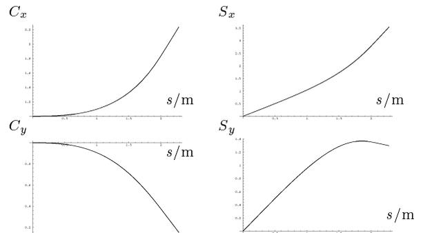
Figure 9: Principal trajectories  $C_x(s)$ ,  $S_x(s)$ ,  $C_y(s)$  and  $S_y(s)$ .
