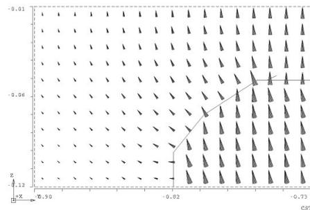
Figure 5: Fringe field at the exit face of the ESR-Dipole with the Rogowski profile.
