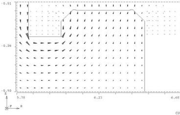
Figure 6: Radial cut which shows the lateral fringe fields, the position of the coils and the shims of the ESR-Dipole.
