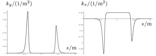
Figure 3: The left plot shows the stiffness parameter  $k_y(s)$  which is proportional to the first order field derivative.  $k_x(s)$  on the right side gives the quadratic path curvature  $h(s)$  minus  $k_y(s)$ . Both parameters are functions of the arc length  $s$ .
