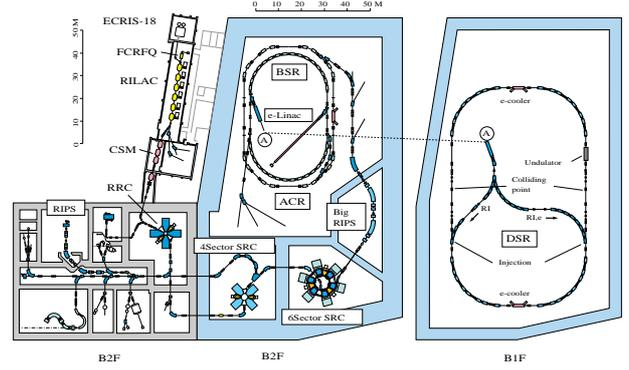
Figure 1: Preliminary layout of the MUSES. The accelerators are housed in the 2-story building.
