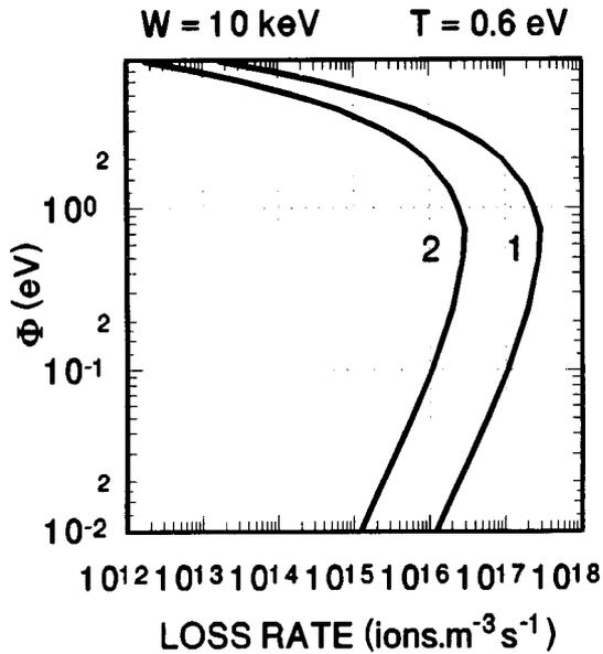
Figure 5: Beam potential  $\Phi$  as a function of loss rate of protons for two different pressures  $p$  into the beam chamber (1:  $p = 10^{-1}$  Pa, 2:  $p = 10^{-2}$  Pa) at the electron temperature  $T = 0.6$  eV and at the energy of protons  $W = 10$  keV.
