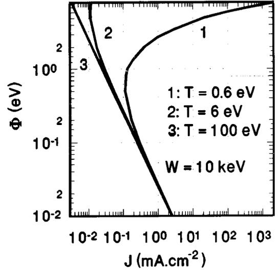
Figure 1: Beam potential  $\Phi$  as a function of mean current density  $J$  for three different electron temperatures  $T$  ( $T = 0.6, 6$  and  $100$  keV) at energy of protons  $W = 10$  keV.
