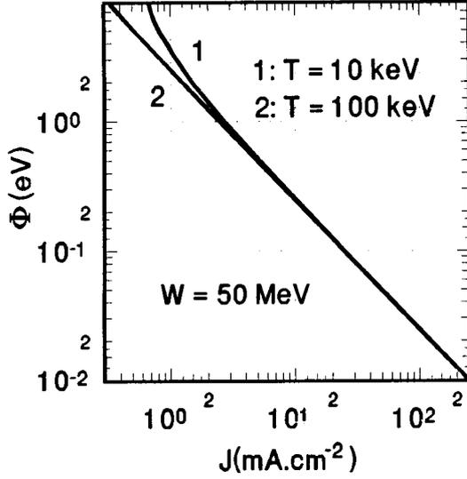
Figure 2: Beam potential  $\Phi$  as a function of mean current density  $J$  for two different electron temperatures  $T$  ( $T = 10$  and  $100$  keV) at energy of protons  $W = 50$  MeV.
