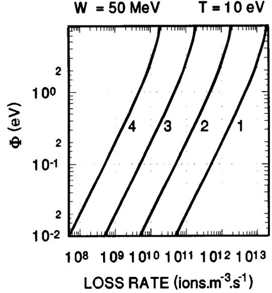
Figure 3: Beam potential  $\Phi$  as a function of loss rate of protons for four different pressures  $p$  into the beam chamber (1:  $p = 10^{-1}$  Pa, 2:  $p = 10^{-2}$  Pa, 3:  $p = 10^{-3}$  Pa and 4:  $p = 10^{-4}$  Pa) at the electron temperature  $T = 10$  eV and at the energy of protons  $W = 50$  MeV.
