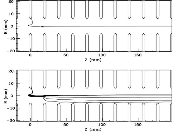
Fig. 3 An example of trajectories which indicates chaotic behaviour. The initial RF phase is changed by  $0.1^\circ$  step in the lower plot.
