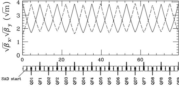
Fig. 1 Accelerator line configuration used in the SAD tracking. The rectangles represent accelerating structures.
