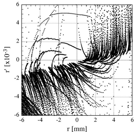
Fig. 4 The distribution in the final phase space with initial position and RF phase changed by  $50 \mu\text{m}$  and  $2^\circ$  step, respectively.
