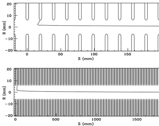
Fig. 2 An example of the trajectory of an electron. The upper plot shows the first 10 cells and the lower shows the whole structure.
