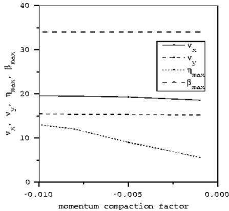
Figure 3: Lattice functions vs. momentum compaction factor.
