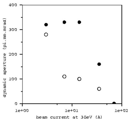
Figure 7: Dynamic aperture with space charge effects.
