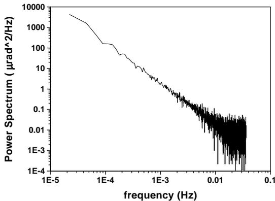
Figure 7: Spectral density obtained in the granite tunnel.
