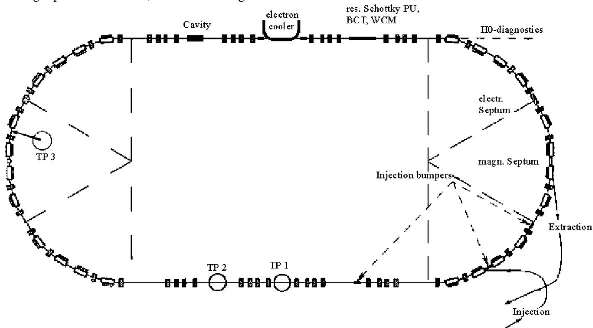
**Fig 1:** Floorplan of the COSY-Ring. Unit cells are indicated. At the places TP1 - TP3 experiments are installed. Some characteristic devices are labelled.
