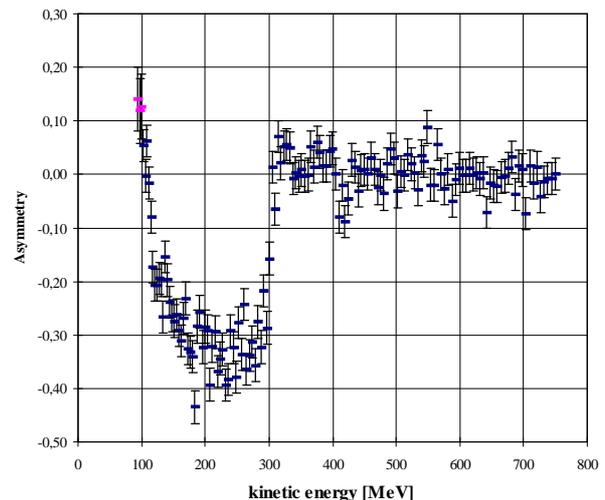
**Fig. 3:** Asymmetry during the acceleration in COSY as recorded by the EDDA detector. The first depolarizing resonance (imperfection) is enhanced to produce a spin flip, the second one (intrinsic) is not compensated. The data shown are raw data.
