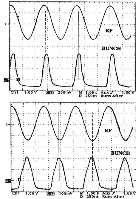
Fig 4: RF and bunch signal before and after shifting transition energy at flat top energy.
