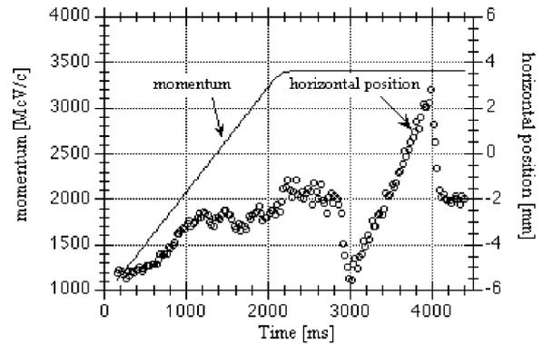
**Fig. 2:** Momentum ramp and horizontal beam position at the EDDA experiment. The special shape of the position curve between 2.6 s and 4.2 s arises from a luminosity check required by the experiment. See text.
