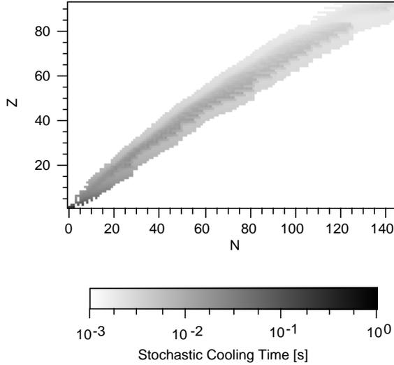
Fig. 2 Similar figure as Fig. 3 except for employing the stochastic cooling. Maximum specifications of the amplifier of 10 kW and 2GHz are assumed in the calculation. The temperature of the pick-up unit is taken as 18 K.
