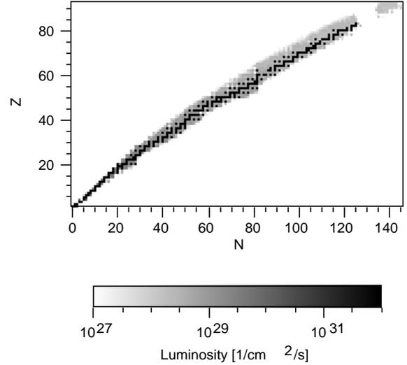
Fig. 5. Luminosity of head-on collision of electrons and unstable nuclei. The length of 10 cm is taken as the interaction region. Dark black squares in the figure represent stable nuclei.
