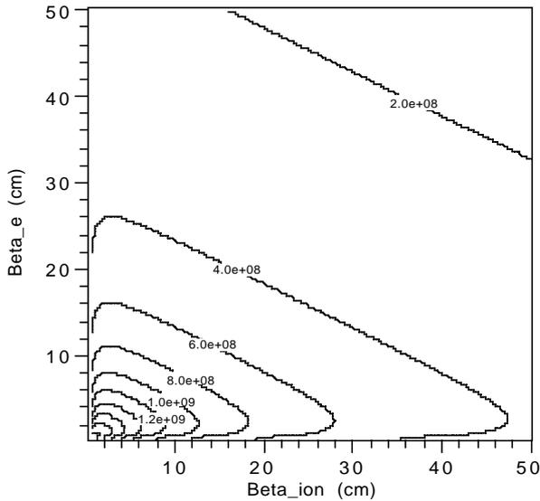
Fig. 4 Contour plot of normalized luminosity. Interaction region of 10cm is assumed in the calculation. Beam emittances are assumed as  $1\pi$  mm mrad for unstable nuclei and  $0.7\pi$  mm mrad for electrons in the calculation.
