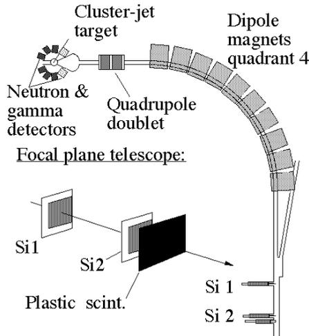
Fig. 2. Schematic picture of an experiment that uses the magnets after the target as a magnetic spectrometer. Si1 and Si2 are silicon strip detectors.
