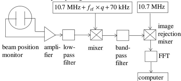
Fig. 1. Simplified schematic of the measurement part of the tune measurement system. The FFT is performed in a digital oscilloscope.
