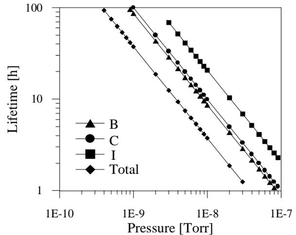
Figure 3. Beam-Gas lifetimes
