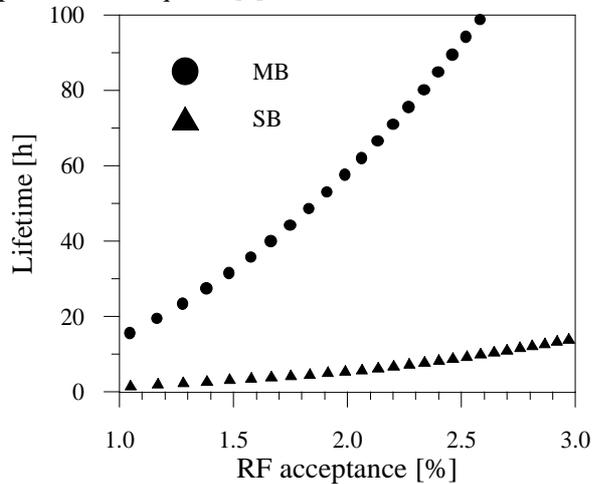
Figure 2. Touschek lifetime for MB and SB operation
