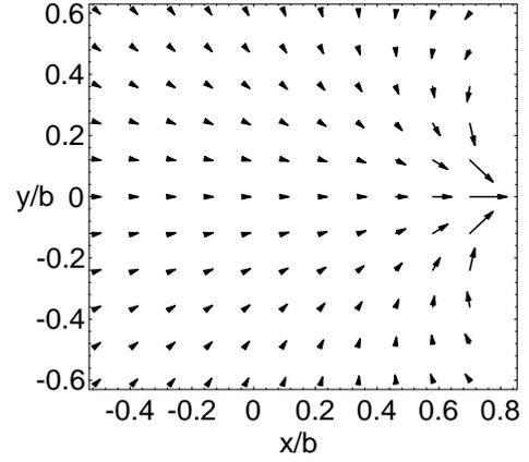
Figure 4: Direction and magnitude of monopole transverse impedance in central region of circular pipe with a hole at  $\varphi_h = 0$  ( $x = b, y = 0$ ) versus beam position, normalized to that magnitude for an on-axis beam.
