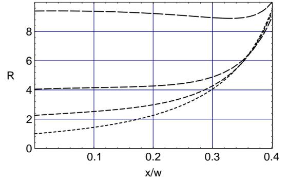
Figure 3: Power loss in square pipe versus horizontal beam offset for different vertical beam offsets  $y/h = 0$  (no offset, short-dashed), 0.2, 0.3, and 0.4 (long-dashed).  $R = 1$  corresponds to an on-axis beam.
