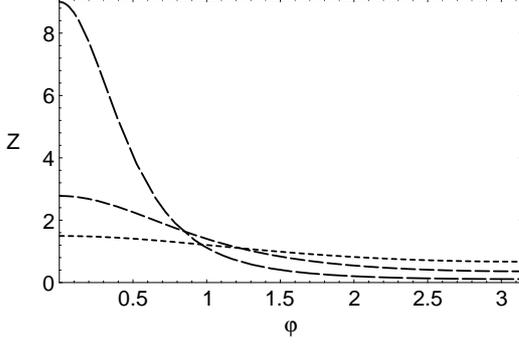
Figure 1: Impedance of a hole in circular pipe versus azimuth angle  $\varphi = \varphi_a - \varphi_h$  between beam and hole (in radians) for different beam offsets  $a/b = 0.1$  (short-dashed), 0.25, and 0.5 (long-dashed).  $Z = 1$  corresponds to  $a = 0$  (on-axis beam).
