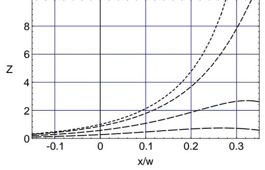
Figure 2: Impedance of a hole in the middle of square-pipe wall ( $y_h/h = 1/2$ ) versus horizontal beam offset for different vertical beam offsets  $y/h = 0$  (short-dashed), 0.1, 0.2 and 0.3 (long-dashed). For an on-axis beam  $Z = 1$ .
