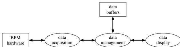
Figure 2: Software structure of the BPM system
