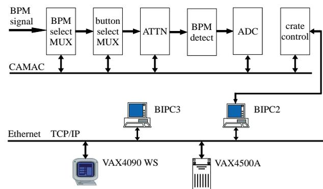
Figure 1: Schematic block diagram of the BPM signal processing electronics
