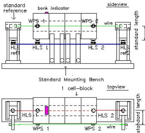
figure 4: cell-block alignment on the bench
