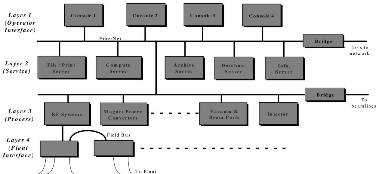
**Figure 1: Proposed Structure of DIAMOND Control System**
