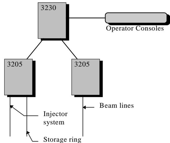
Figure 1: The SRS Control System
