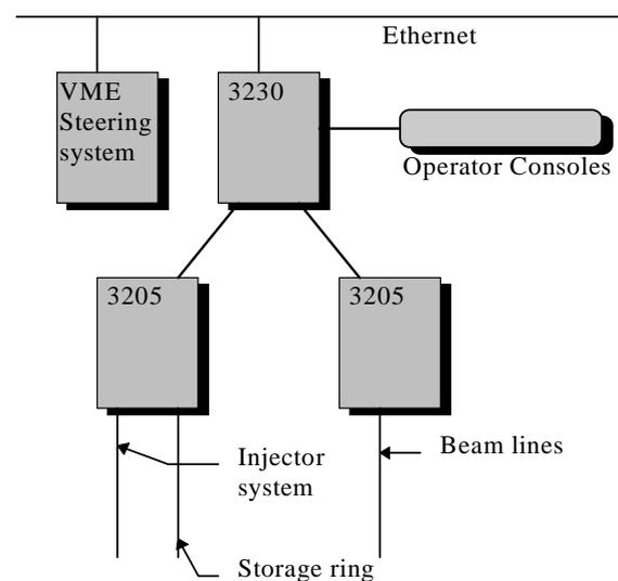
Figure 2: SRS Control System in 1993
