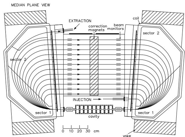
Figure 3: 10–75 MeV racetrack microtron.
