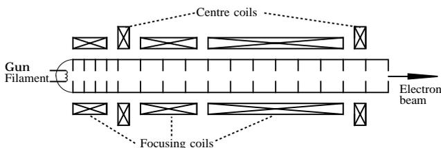
Figure 1: 10 MeV linear accelerator.
