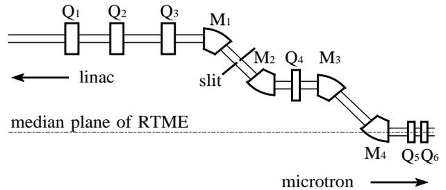
Figure 2: Beamline from LINAC10 to RTME.
