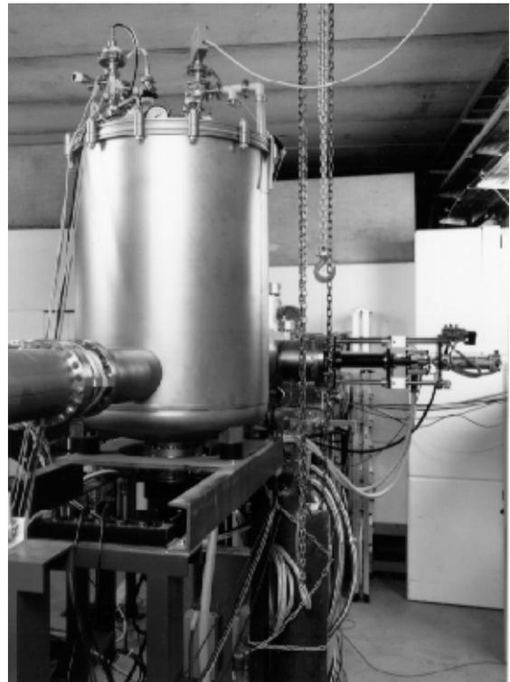
Figure 1: Cryostat with detector system built in the beam line of the beam diagnostics test facility (Photo: Achim Zschau, GSI)
