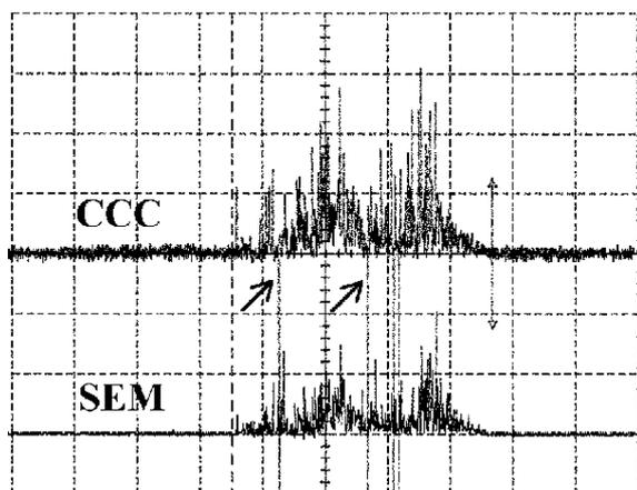
Figure 4: Measured ion current pulse extracted from the SIS; x-axis: 500 ms per div., y-axis: 0.5 V per div. ( $\cong 35.5$  nA ion current per div. for the CCC)
