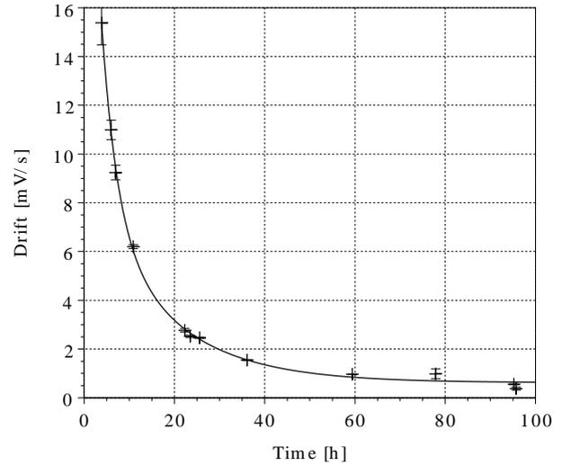
Figure 3: Measurement of the zero drift
