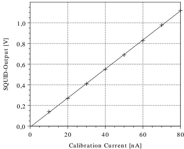
Figure 2: Plot of current calibration data
