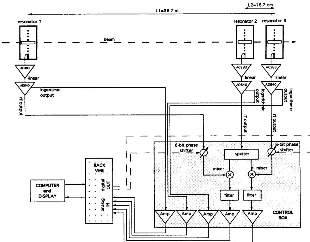
Figure 2: Schematic of the electronics
