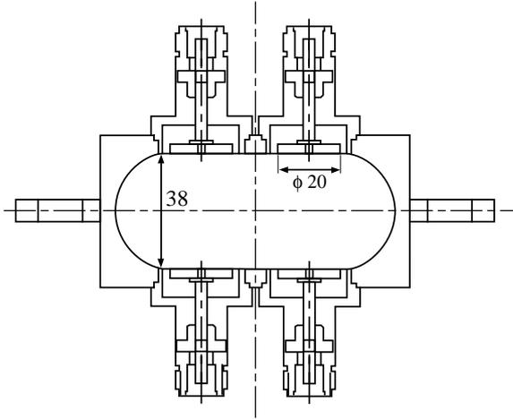
Figure 2 : Cross-sectional view of a BPM at SOR-RING.
