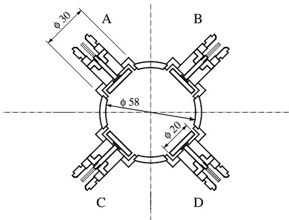
Figure 3 : Cross-sectional view of a BPM at the BT-line.
