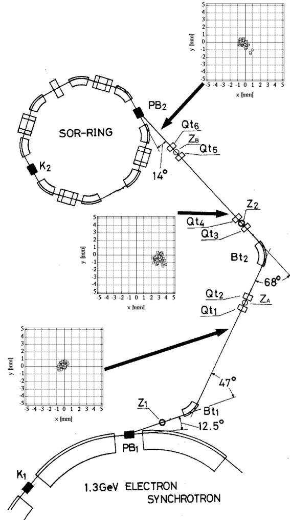
Figure 7 : The schematic view of the BT-line and results of the single-pass monitoring of beam positions.
