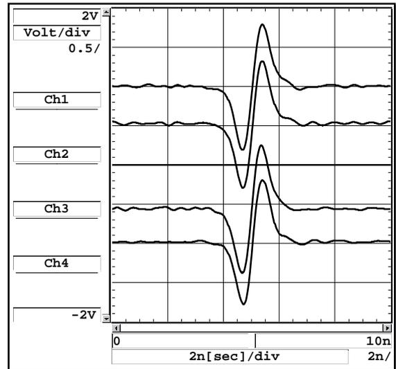
Figure 4 : An example of four button signals of a BPM.
