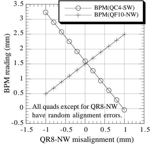
Figure: 1 Estimated beam position monitor readings for  $\kappa=5\%$  for misalignment of a quadrupole magnet (QR8-NW) at two points, 1300 deg upstream (QC4-SW) and 270 deg downstream (QF10-NW) of QR8-NW. All quads have random alignment errors in addition to the fixed error of QR8-NW quad.
