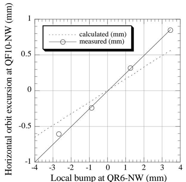
Figure: 4 Comparison between the orbit measurement and calculation for a quad (QR6-NW). Shunt current (10A) is 3% at injection field.
