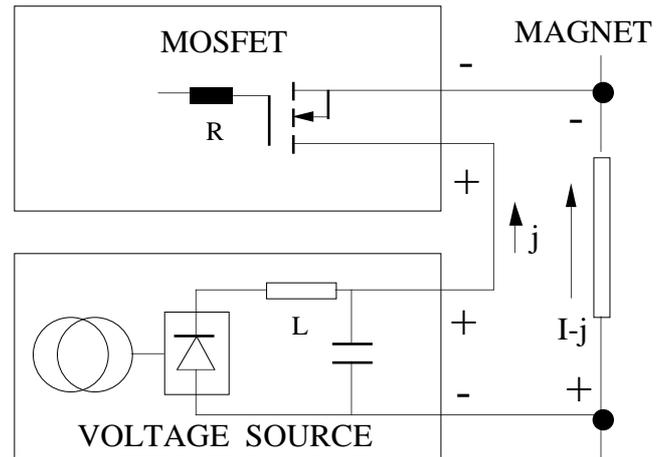
Figure: 3 Voltage source to feed the forced reverse current to the magnet. It produces compensation voltage to the FET shunt of Fig.2 when used at lower terminal voltage.
