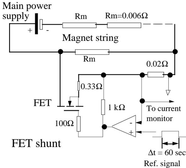
Figure: 2 Simplified model circuit of the FET current shunt.
