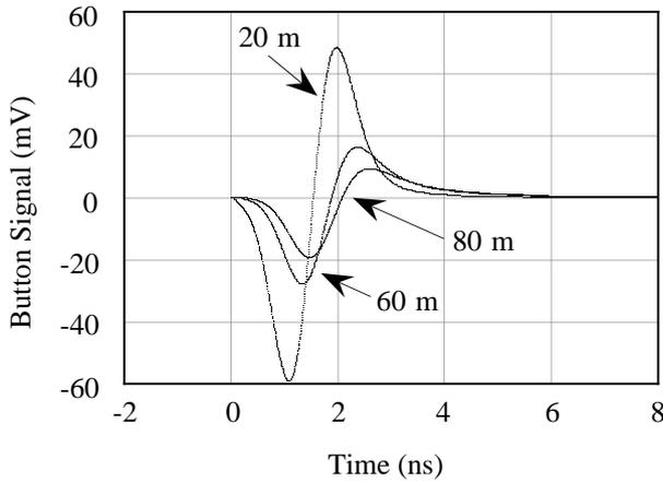
Figure 2 Simulation of the signal attenuation in the coaxial cable.
