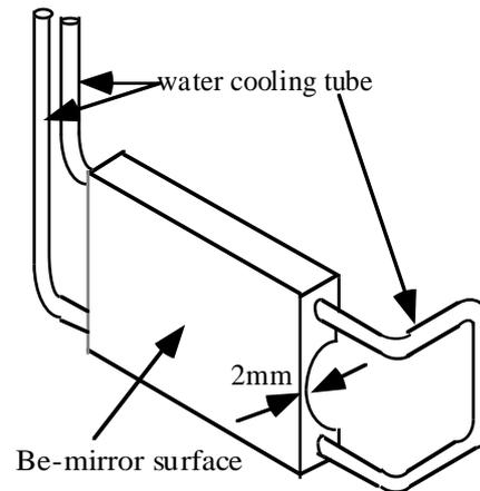
Figure 1 Design of the Be-mirror.
