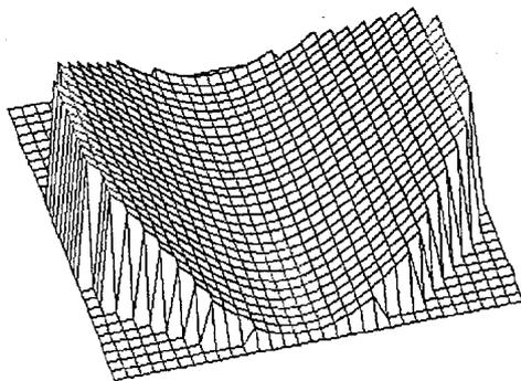
Figure 2. Surface deformation caused by  $150^{\circ}$  C baking. The side length of three dimensional plot is 50mm
