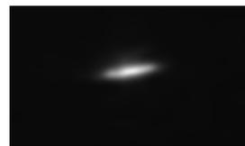
Fig. 5 Beam profile after deconvolution process, scale is same as in Fig.4.
