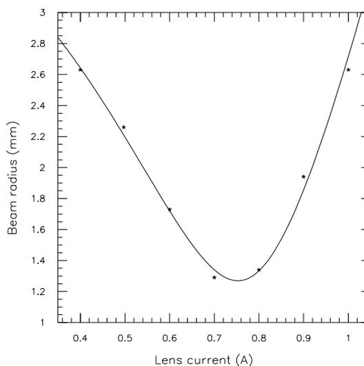
Figure 3: Beam dimensions vs lens intensity
