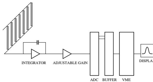
Figure 1: Block diagram of the SEM-Grid Electronics
