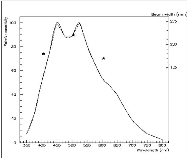
Fig. 4. Spectral response of the intensified camera. The experimental measured widths are superimposed.
