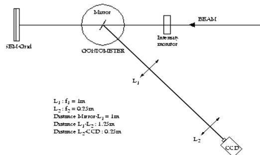
Fig 1. The experimental set-up
