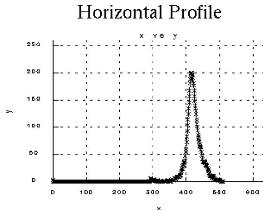
Fig. 3. Beam profile for 500nm wavelength. Camera gain = 125.
