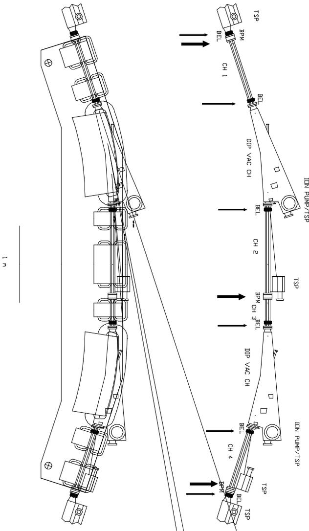
Fig. 2. The vacuum system of one ring cell. The thin arrows show the locations of bellows and the thick arrows the location of BPM heads.
