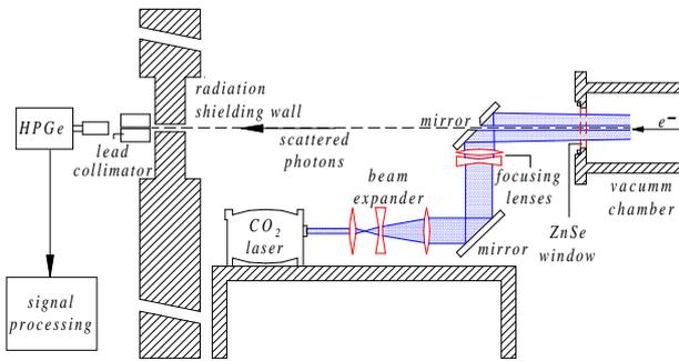
**FIG. 1** Schematic diagram of the overall system: part of the vacuum chamber of the storage ring, optical system, detecting system, and signal processing system.
