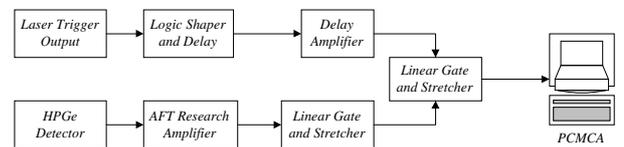
**FIG. 2** Instruments associated with synchronous measurement.
