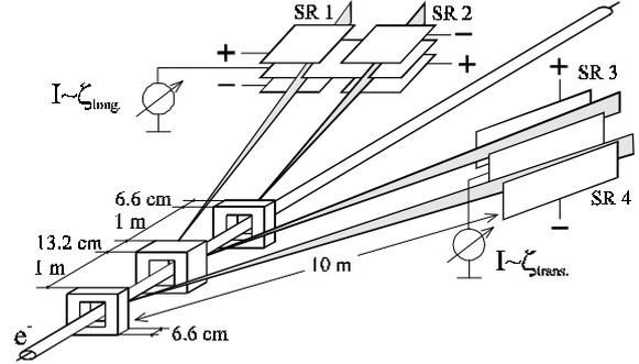
Figure 3. The schematic view of vector polarimeter.
