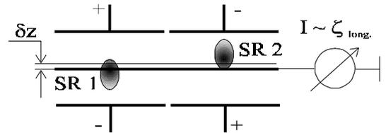
Figure 1. Compensation of SR beams vertical displacement,  $\delta z$ , by four electrodes DIC.
