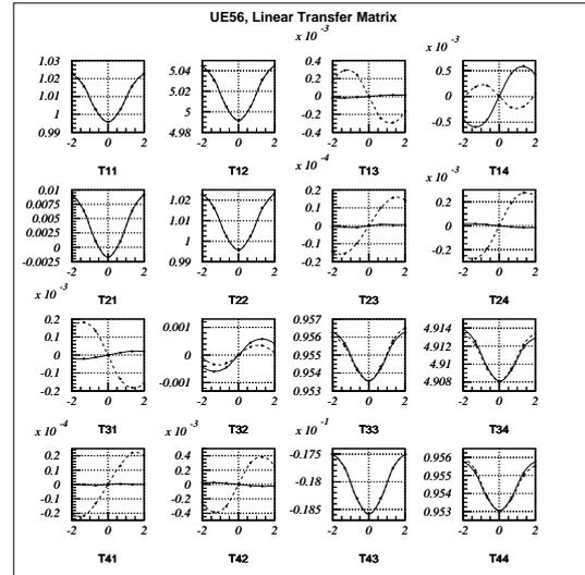
Figure 4: The sixteen plots show the elements of the linear transfer matrix of the elliptical undulators as a function of the phase shift i.e. row shift. The solid lines refer to the case where both undulators have the same helicity, the dashed lines refer to an opposite helicity.
