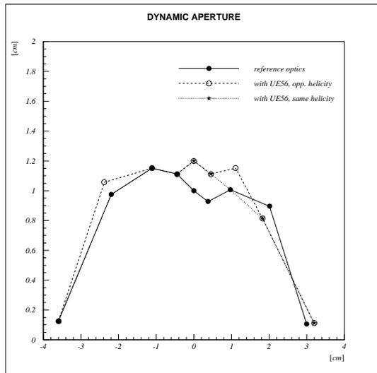
Figure 5: The figure shows the dynamic apertures for the reference optics with a standard set of insertion devices and the optics including an UE56 (two modules).
