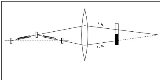
Figure 1: Setup of the double elliptical undulator and a chicane to separate the two beams, which are focussed to a probe.
