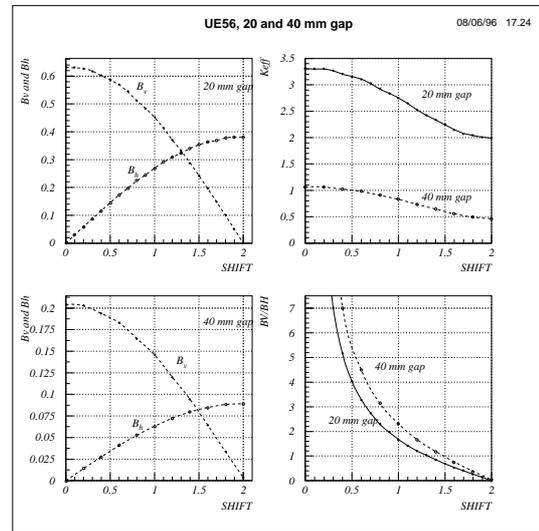
Figure 2: Dependence of horizontal and vertical field components  $B_h$  and  $B_v$ , respectively, and the resulting K-value for two different gaps on the shift parameter.
