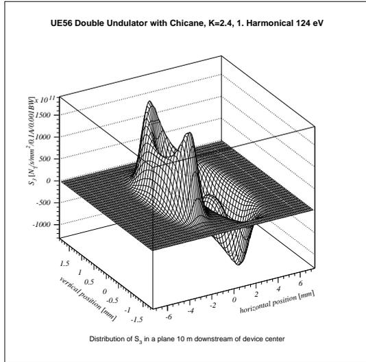
Figure 3: The figure shows the circularly polarized photon flux density  $S_3$  in a 10 m distance from the center of the straight section. The spererated cones corresponds to the left and right handed light of the two elliptical undulators.
