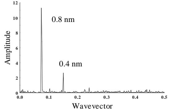
Fig.4 Longitudinal charge density Fourier analysis
