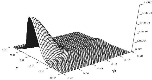
Fig.3 Angular and Spectral distribution of radiation in joules per steradian.
