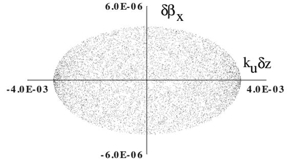
Fig.1 Initial  $x$ - $\beta_x$  phase space of 5000 particles
