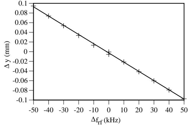
Figure 1. Typical measurement of vertical orbit change with RF frequency.
