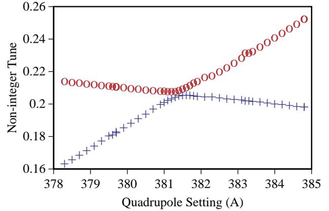
Figure 5. Variation of the radial and vertical betatron tunes with quadrupole setting.
