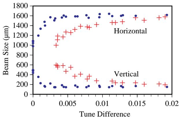
Figure 8. Beam size as a function of tune difference for low coupling orbit (•) and standard orbit (+).
