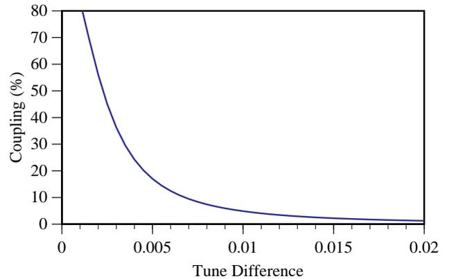
Figure 6. Variation of coupling with tune difference near the resonance  $Q_r - Q_v = 1$ .
