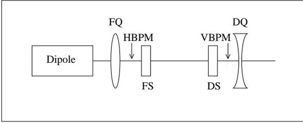
Figure 3. Schematic of the SRS unit cell.
