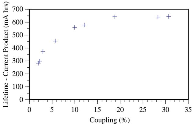
Figure 7. Variation of lifetime-beam current product as a function of coupling ratio.
