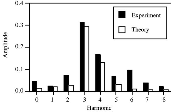
Figure 4. Theoretical and experimental Fourier transform of the vertical dispersion.
