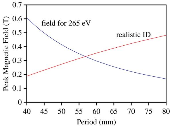
Figure 2. Plot showing the peak magnetic field required to reach 265 eV with the first harmonic and the realistic fields achievable from an APPLE type device.
