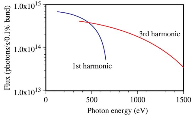
Figure 6. Undulator tuning curve.
