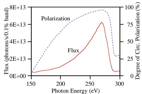
Figure 7. Integrated flux and degree of circular polarization for minimum gap condition. Beamline aperture is 0.2 mrad x 0.2 mrad square aperture.
