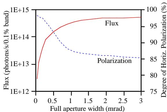
Figure 5. Flux and degree of horizontal polarization in the first harmonic through a square aperture at  $K_v = 1.5$ .
