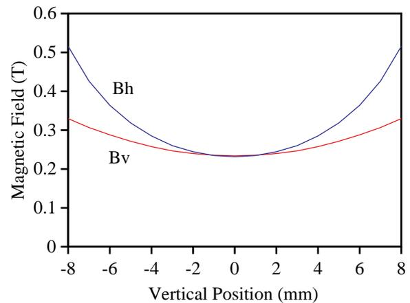
Figure 4. Horizontal and vertical magnetic fields along the y-axis assuming the arrays touch each other.
