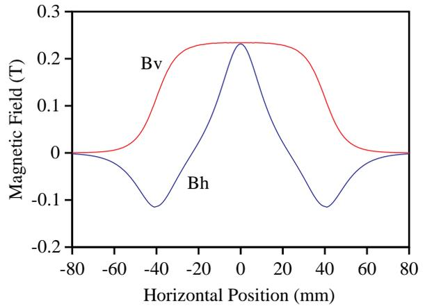
Figure 3. Horizontal and vertical magnetic fields along the x-axis assuming the arrays touch each other.
