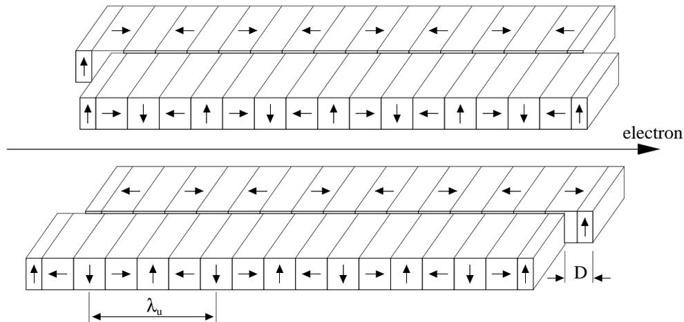
Figure 1. Sketch of the Planar Helical Undulator
