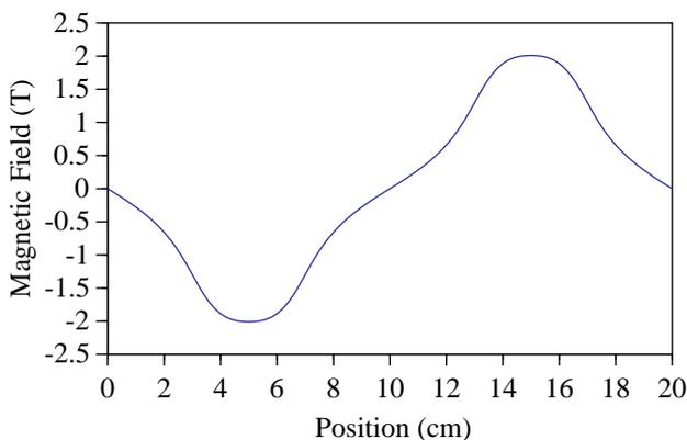
Figure 2. Magnetic field variation for one period of the proposed MPW.
