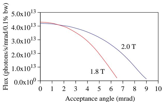
Figure 1. Photon flux vs horizontal acceptance angle for two MPW designs at 10 keV.
