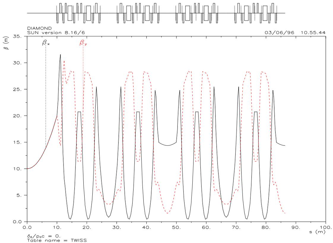
Fig 1: Beta functions around one quarter of DIAMOND
