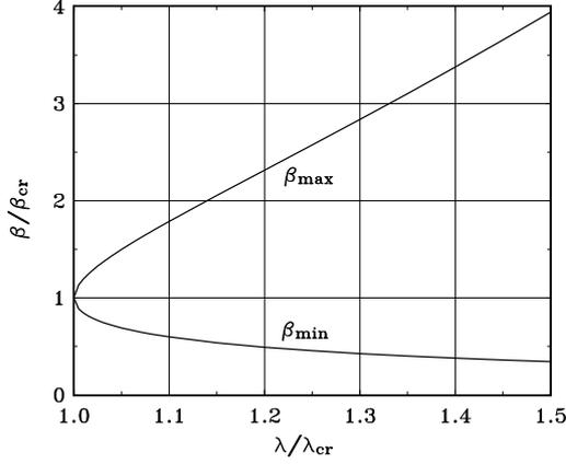
Figure 1: Safety limits for the external beta function versus the radiation wavelength.
