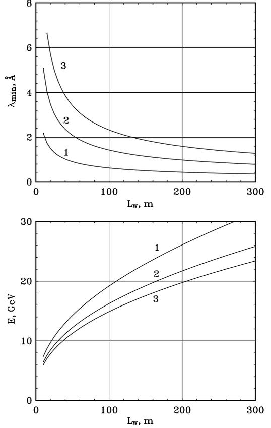
Figure 2: Minimal achievable photon wavelength in an FEL amplifier and corresponding energy of the electron beam versus the length of the undulator  $L_w$ . The curves 1, 2 and 3 correspond to values of the normalized emittance  $10^{-4}$  cm rad,  $2 \times 10^{-4}$  cm rad and  $3 \times 10^{-4}$  cm rad, respectively. The energy spread at the entrance of the undulator in all cases is equal to  $\sigma_{E0} = 1$  MeV.
