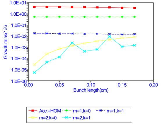
Figure: 3 Growth rates and bunch length for the several modes.
