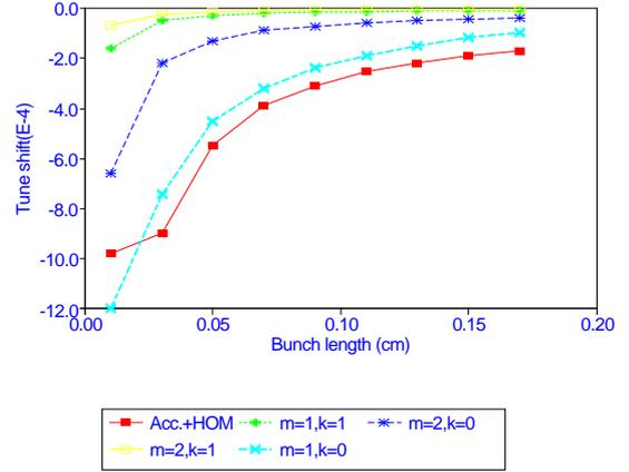
Figure: 4 Tune shift and bunch length for the several modes.
