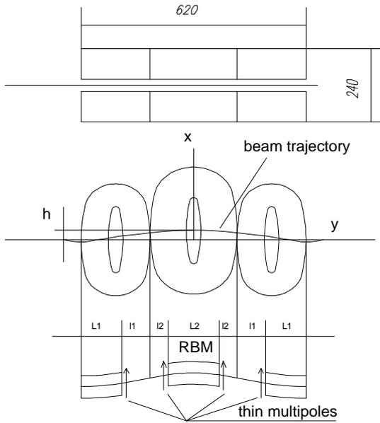
Fig.1. The wiggler diagram. RBM - rectangular bending magnets, h - the shift of the principal pole.
