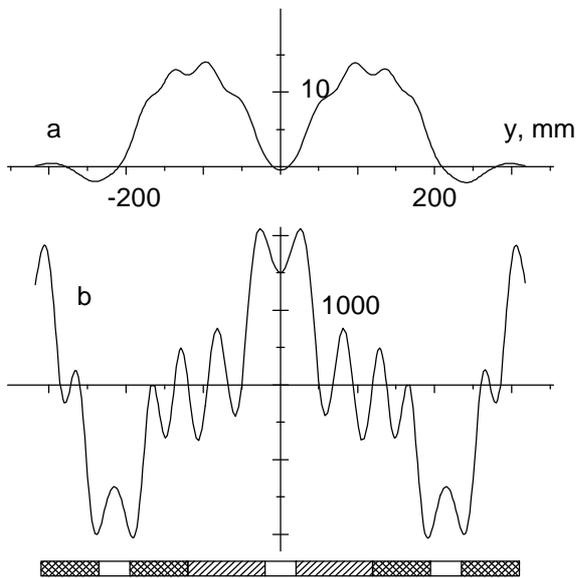
Fig.2 The distribution of the quadrupole and multipole components of the wiggler field:
