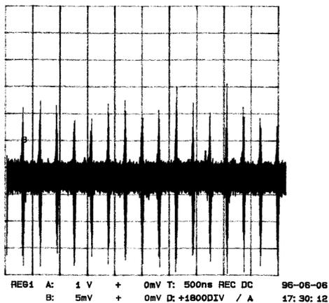
Figure 3: Observation of 3000 turns detected by the beam position monitor AMP06. Time delay is 1 millisecond.
